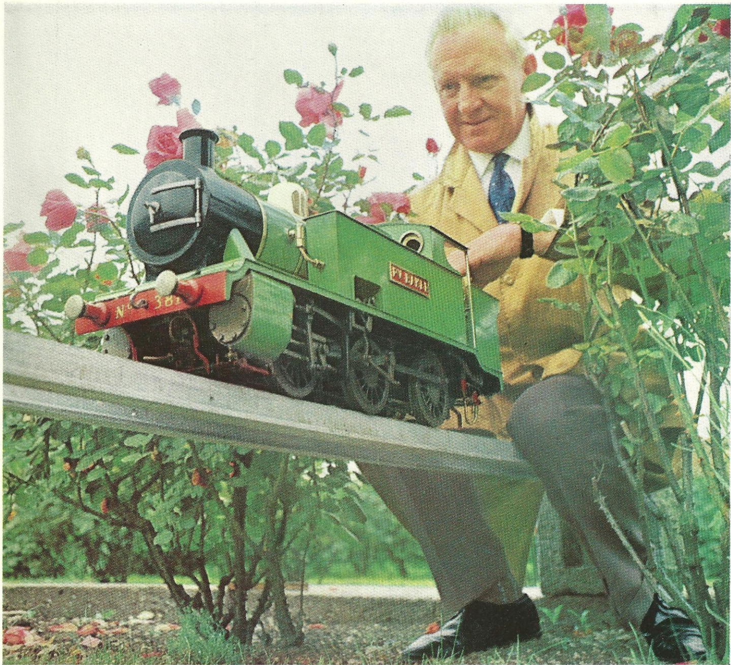
The P. V. Baker, a 0-6-0 tank engine, has a gauge of 3\frac{1}{2} in. and runs on coal at a working pressure of 80 lb. sq. in. It can pull four men.
